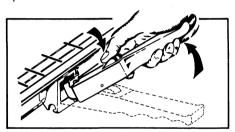
When grilling, the grill pan is placed on the shelf, ensuring that the cut out on the underside of the handle bracket locates over the front edge of the shelf.
